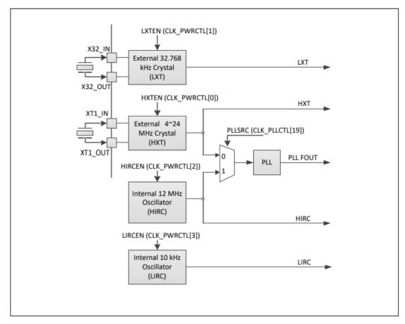
Figure 4.3-3 Clock Generator Block Diagram
