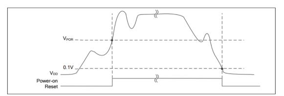
Figure 4.2-3 Power-on Reset (POR) Waveform
