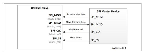
Figure 4.26-2 SPI Slave Mode Application Block Diagram
