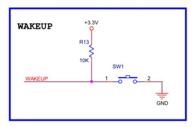
To test this example, wire a pushbutton to your ITM-MV8 series module by following the schematic diagram. The button is connected to PC.0 (Wakeup pin) using a pull high 10k Ohm resistor.
