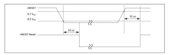
Figure 4.2-2 nRESET Reset Waveform
