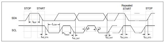
Figure 4.27-1 I<sup>2</sup>C Bus Timing
