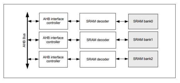
Figure 4.2-9 SRAM Block Diagram
