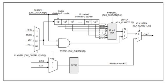
Figure 4.3-7 Clock Output Block Diagram
