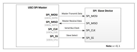
Figure 4.26-1 SPI Master Mode Application Block Diagram
