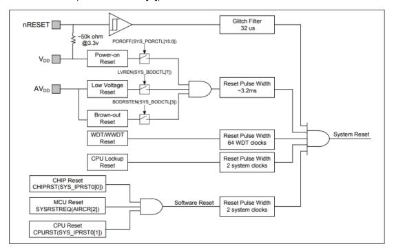
Figure 4.2-1 System Reset Sources
