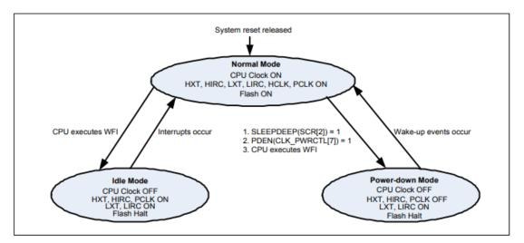
Figure 4.2-7 Power Mode State Machine
