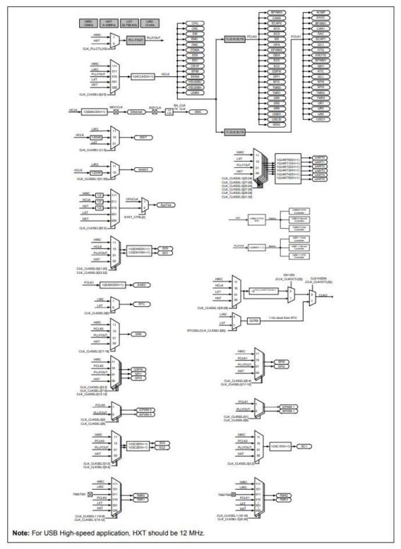
Figure 4.3-1 Clock Generator Global View Diagram (ITM-MV8)
