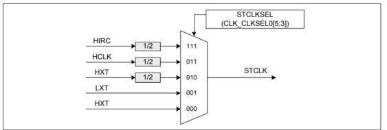
Figure 4.3-6 SysTick Clock Control Block Diagram
