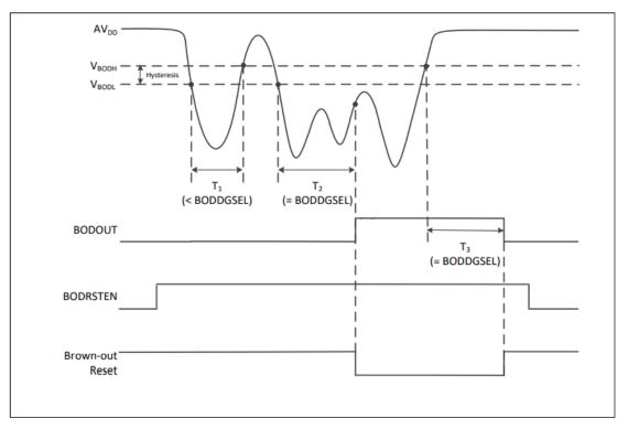
Figure 4.2-5 Brown-out Detector (BOD) Waveform
