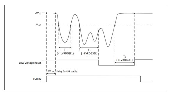
Figure 4.2-4 Low Voltage Reset (LVR) Waveform
