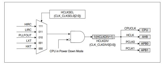
Figure 4.3-4 System Clock Block Diagrams
