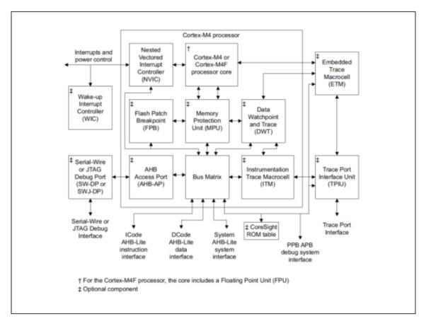
Figure 4.1-1 Cortex®-M4F Block Diagram
