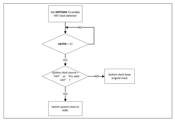
Figure 4.3-5 HXT Stop Protect Procedure
